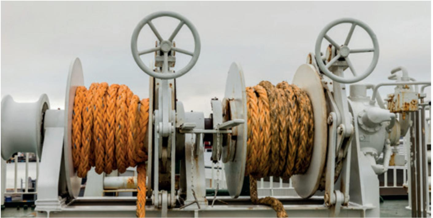
Any rope that has been in use for any period of time will show signs of wear and tear, some characteristics of use will not reduce strength while others will. Ropes should be inspected on a regular basis for wear and tear and any faults / repair / retirement required.
